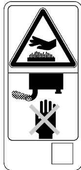
(3) Part No. 6F172-4719-3 Do not touch hot surface like muffler and so on.
