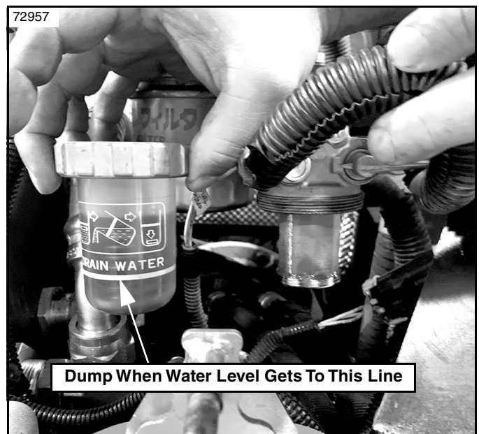
Sediment Cup Drain Line Figure 5-10
