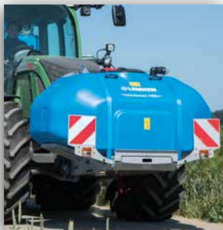
Gemini front tank with 1,100 l capacity
