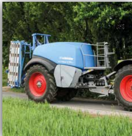
Low centre of gravity due to compact, rear-folding SEH boom
