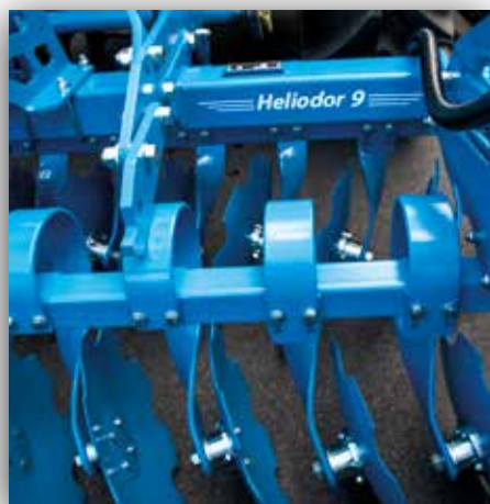
Separately adjustable discs in the tractor track
