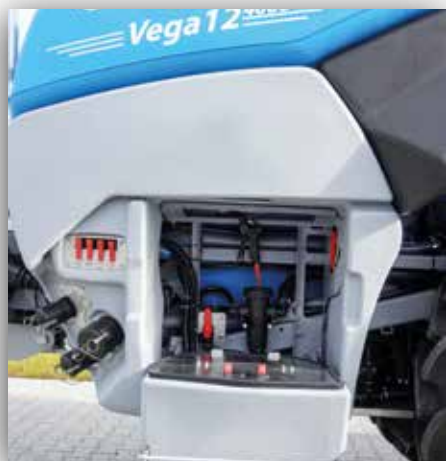
Optimally integrated inductor with electronic operating centre
