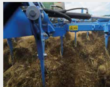
4 rows of tines for intensive mixing
