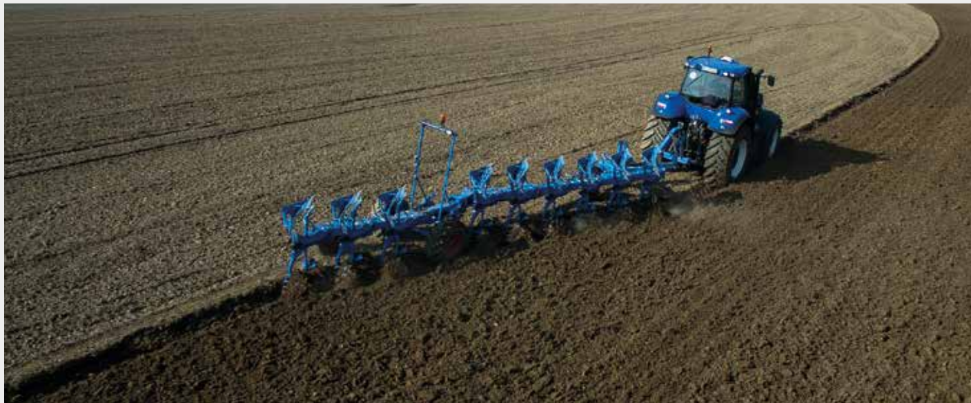
The new LEMKEN Titan 11 with Hydromatic hydraulic overload protection
