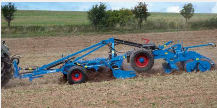
Karat cultivator with working depth control ContourTrack
