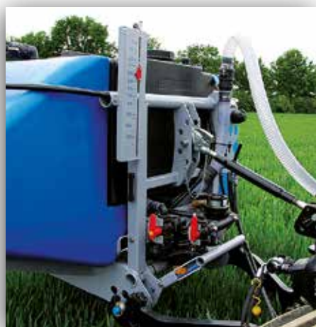
Special mounting frame, shallow design
