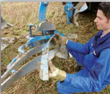
LEMKEN DuraMaxx parts can be changed quickly without tools
