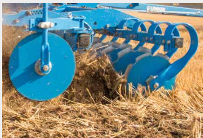
Serrated concave discs for intensive mixing
