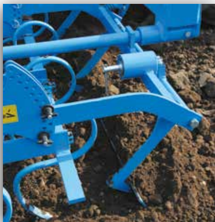
Working action of the levelling bar
