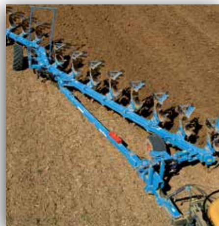
Front support wheel inside the plough frame
