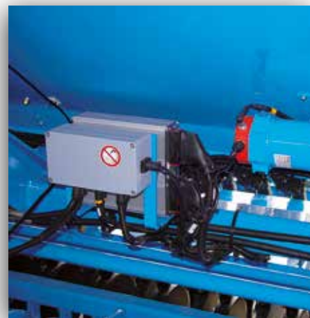
The electric seeding shaft drive
