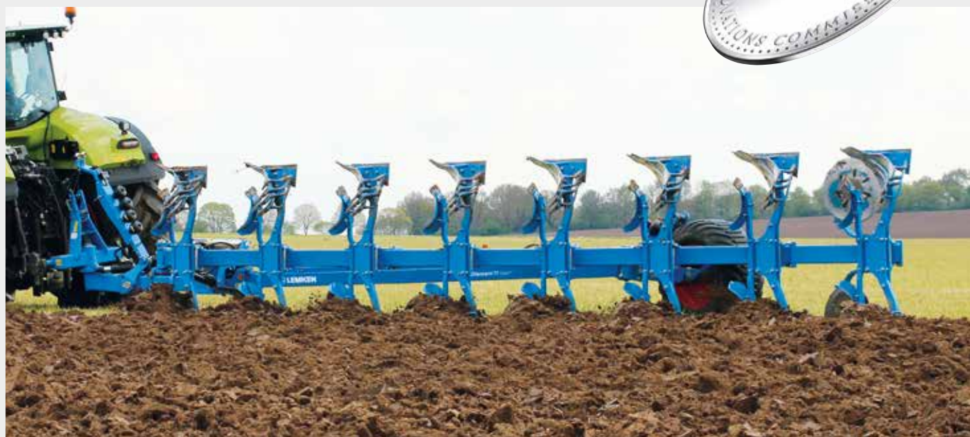
Semi-mounted reversible Diamant plough with OptiLine adjustment system
