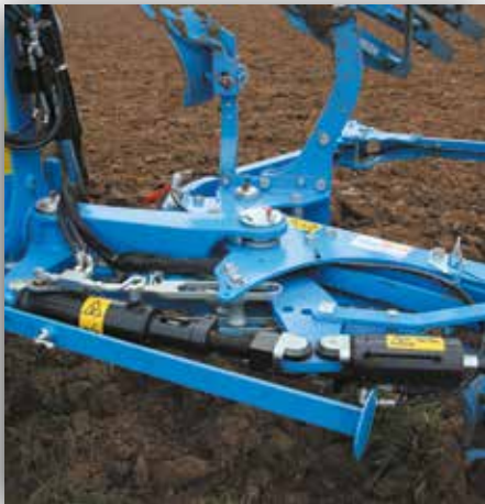
Hydraulic ram for working width adjustment
