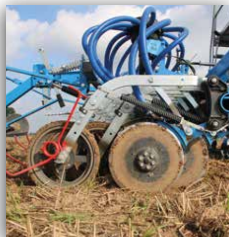
The double disc coulters OptiDisc mechanical up to 45 kg coulters pressure
