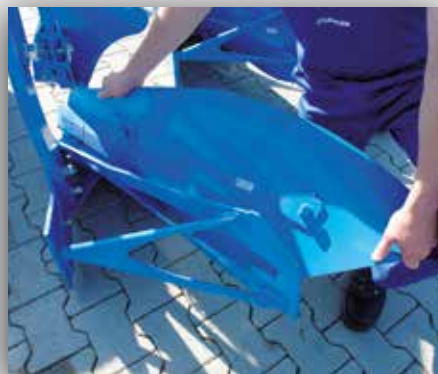
LEMKEN DuraMaxx mouldboards and slats are attached with only two hooks
