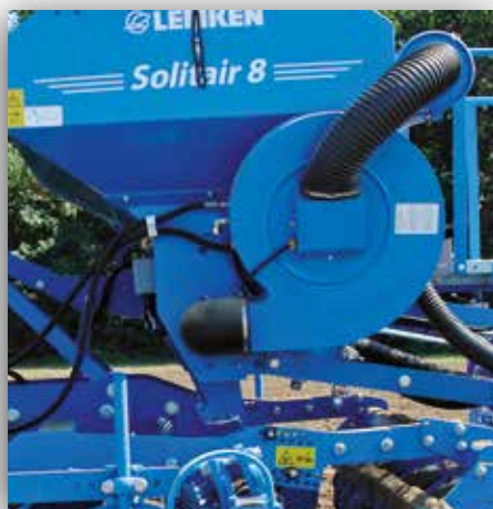
The hydraulically driven fan
