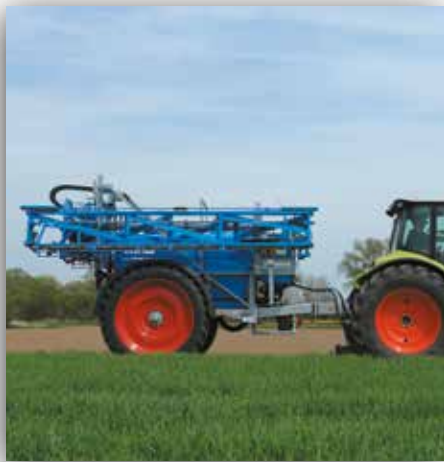
Close coupling ensures sprayer wheels follow tractor wheels as closely as possible
