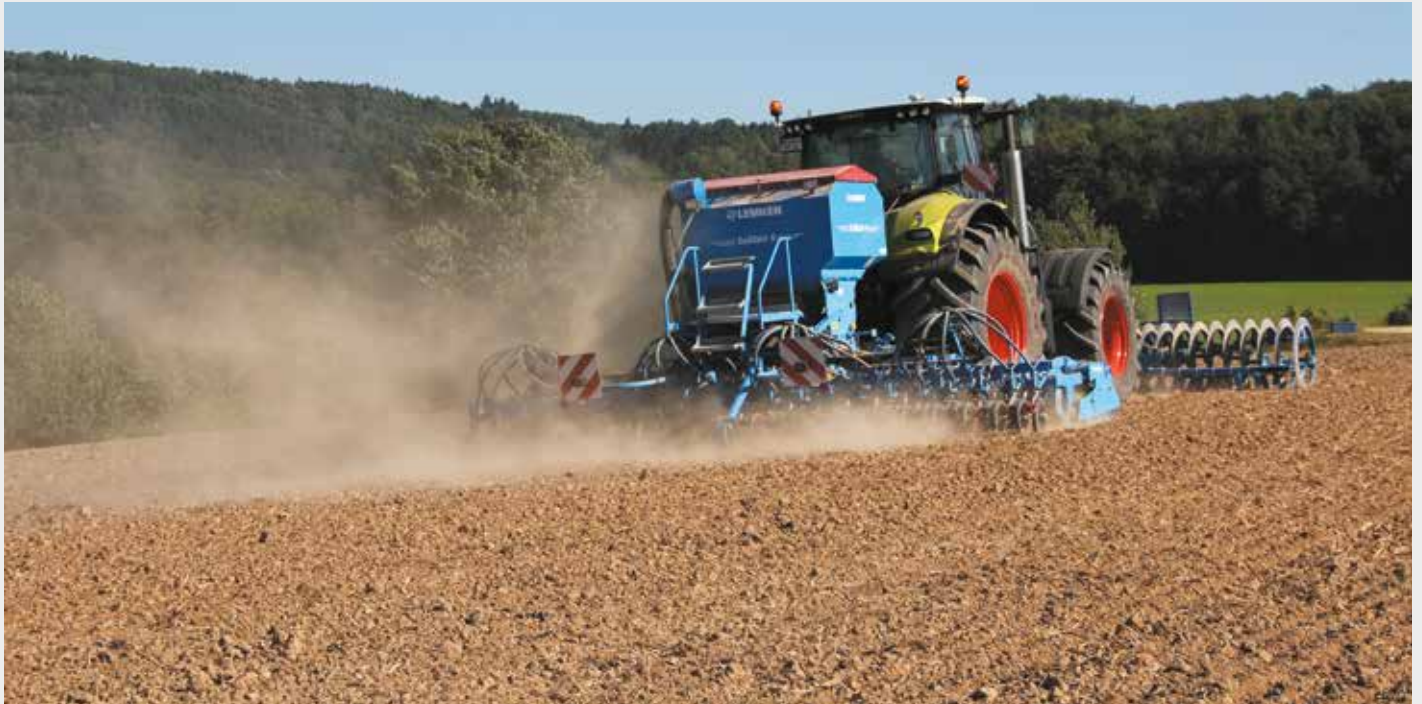
Zirkon-Solitair drill combination with GPS tramline mechanism
