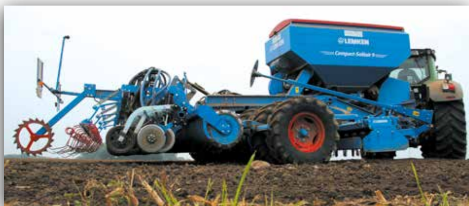
The Compact-Solitair KK with power harrow and six metres working width
