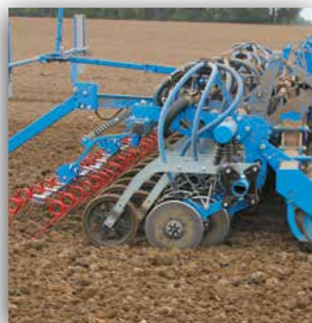
The double disc coulters OptiDisc hydraulic up to 70 kg coulters pressure
