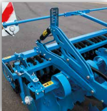
Hydraulic working depth adjustment
