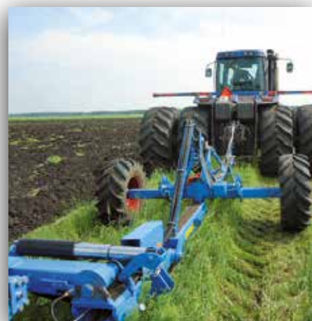
Coupling carriage for tractors without hydraulic three point linkage
