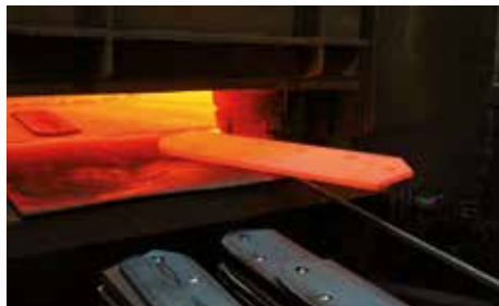
Automated Steel Forming & Tempering System
