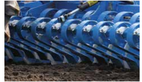
Perfect leveling with leveling work tines
