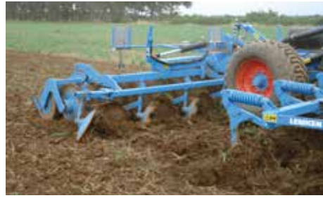
Automatic adjustment of the leveling discs
