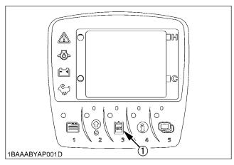
(1) AUX port enable switch (Switch 3)
