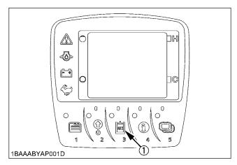
(1) AUX port enable switch (Switch 3)
