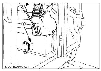
(1) Inlet selector lever (A) "FRESH AIR INLET" position
