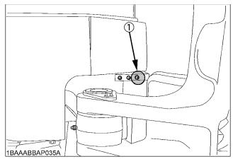
(1) Grease fitting (for swing bearing teeth)
