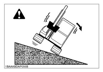
Recommended technique for working on a slope.
