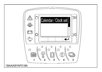
3. Press the switch 5 and the following detailed screen shows up.
