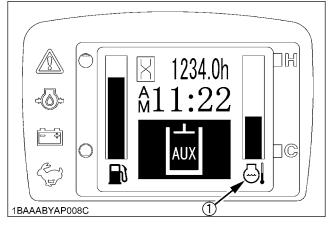
(1) Coolant temperature sensor marker
