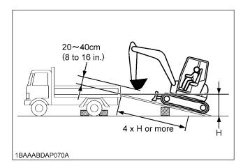
3. For additional safety, use blocks or supports under the ramps and the bed.
