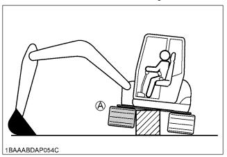
(A) "Rotate to remove sand and gravel"
