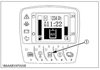
(1) AUX port flow rate limit switch
